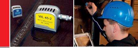
The high precision SONOSCAN probes are manufactured in three different construction types. They can be selected according to their angle, frequency, transducer size and environmental conditions. In addition to standard probes, customer specific solutions can be realized.
